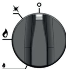
Figure 6. Setting a knob in the position, in which the gas supply to the burner is completely cut off.
